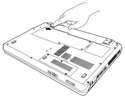
(Sample Illustration) Unlocking the battery release lock
